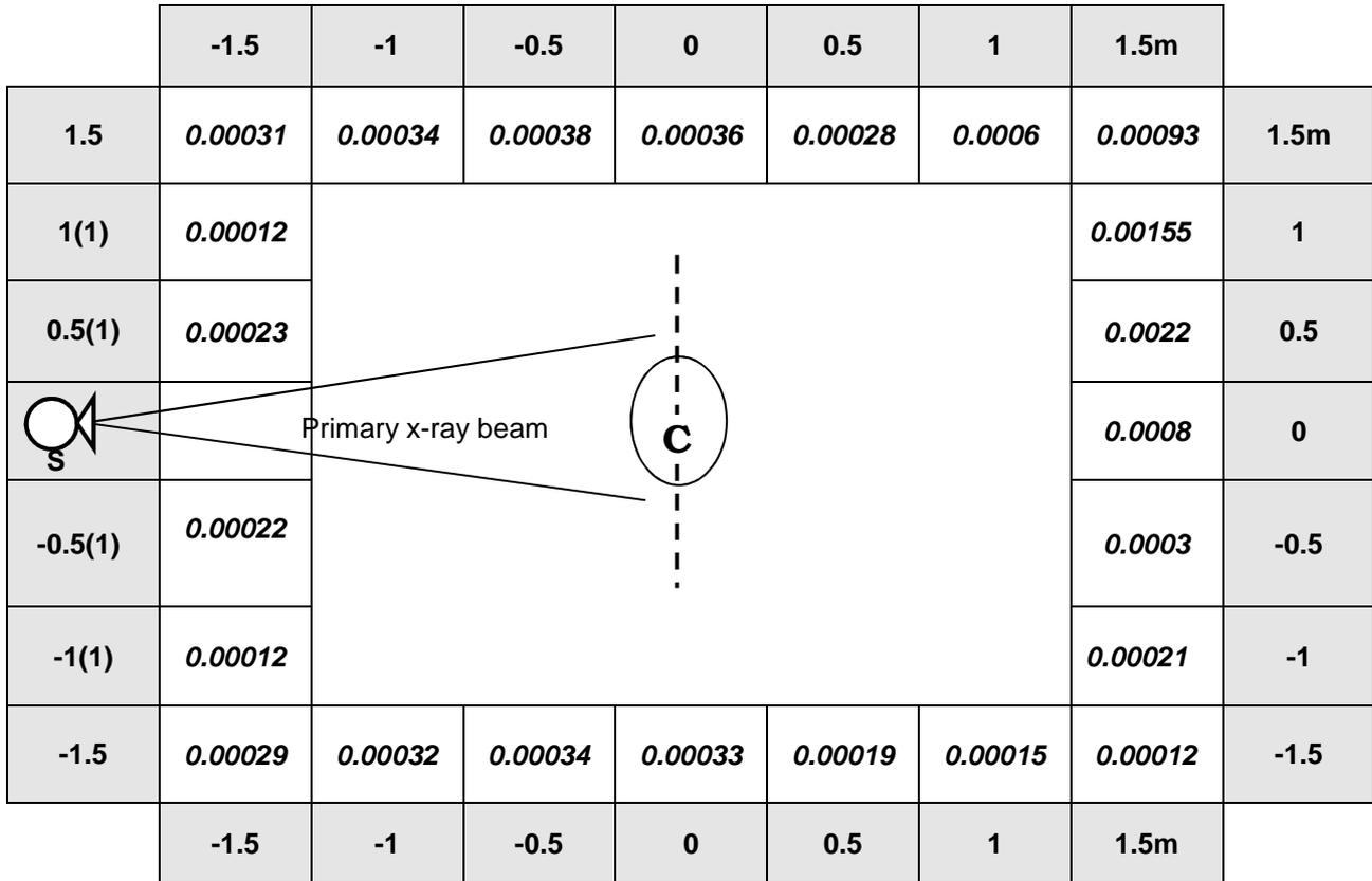
Figure 4: Distribution of stray radiation in Ceph examination
