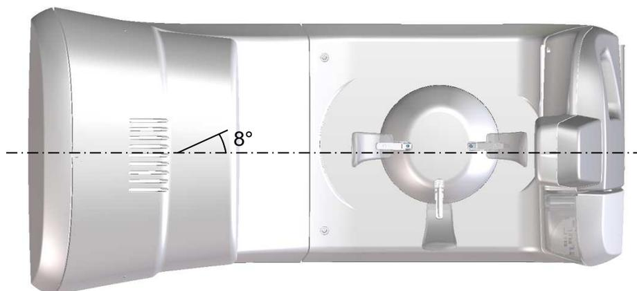
Figure 5 - Tube-head target angle (view from the bottom)
