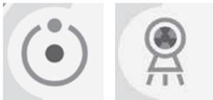
There are two light indicators; the first one on the top indicates the condition "Machine Ready", indicating the user that by pressing the X-ray button key once more, X-rays emission will start; the second indicates the effective emission of X-rays.
