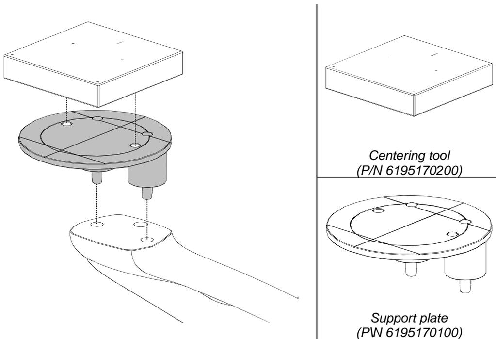
Figure 8: Support plate and centering tool positioning
